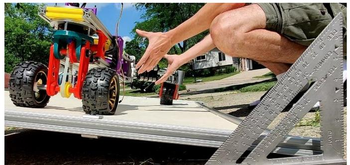
**Figure 15:** Experimental Tilt Test (Prior to Leg Reinforcement)
