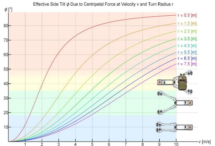
**Figure 16:** Effective Side Tilt Experienced During Turning Maneuvers
