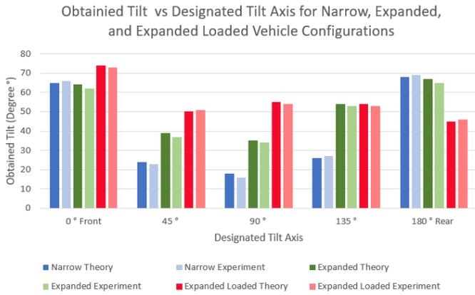
**Chart 1:** Tilt Orientation vs. Obtained Tilt Degree for Narrow, Expanded, and Expanded Loaded Configurations
