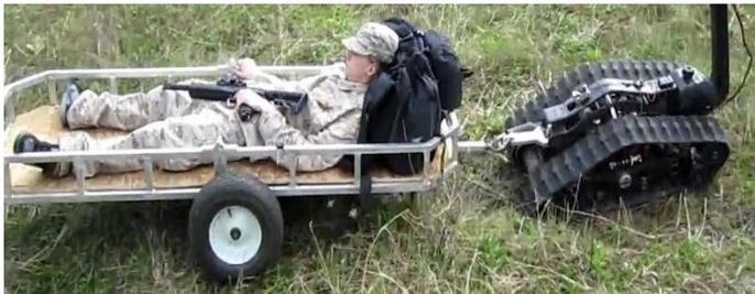
**Figure 4.** DTV Shredder Personal Tracked Vehicle in the Medical Evacuation Role [15]
