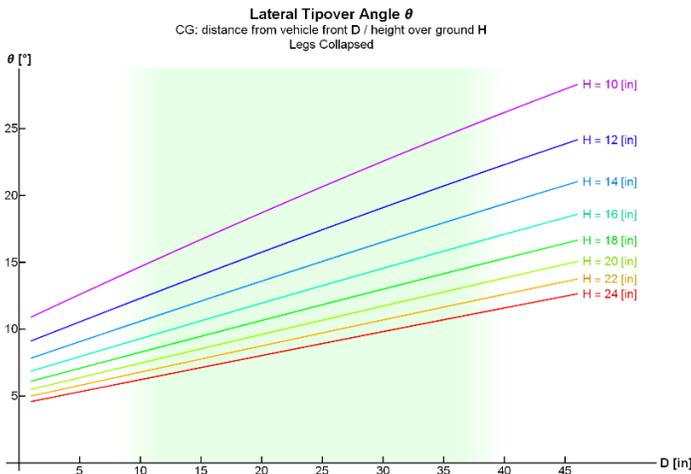
**Figure 18:** Lateral Tip over Angle Theta in terms of Distance **D** from Vehicle front over ground Height **H** Legs Narrow
